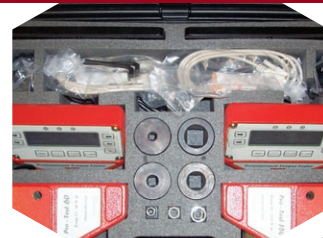
Military Torque Wrench Tester Kit containing two instruments giving a total calibrated range from 1.2 to 1500 Nm. NATO stock number 6635-99-511-0355.
